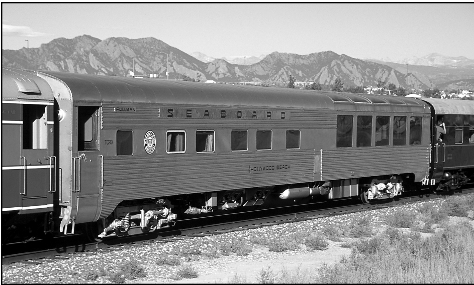
HOLLYWOOD BEACH (SCL #20) joined the Seaboard Air Line RR in January 1956. Pullman-Standard lot 6970, plan 4202 was this 6-double bedroom-bar-sun lounge car. It passed the Flatirons west of Broomfield, CO, on BNSF's Front Range Subdivision on 9/18/04. – Photo © Chip 2004.
